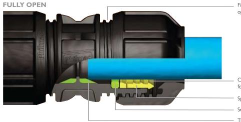
Fitting is pre-assembled ready to use in the open position with 2 threads showing.
