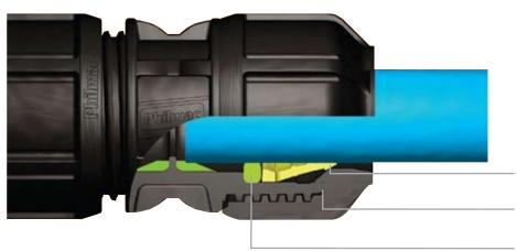
Split collet bites into the pipe providing end load resistance.
